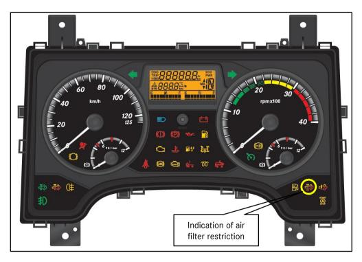
Air filter restriction indication on instrument cluster
