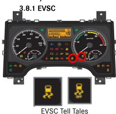
The 917/1017 RHD chassis are supplied with **Electronic Vehicle Stability Control System (EVSC)**, as mandated by the "AIS-150" and should be fixed in the Body/chassis Post bodybuilding the following recommendation's are to be followed to ensure proper integration of the EVSC system.
